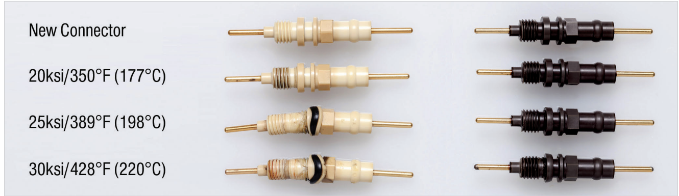
PEK connector rated to 20 ksi/400°F (1,379 bar/204°C) (left), Arlon® 3000 XT connector (right)
